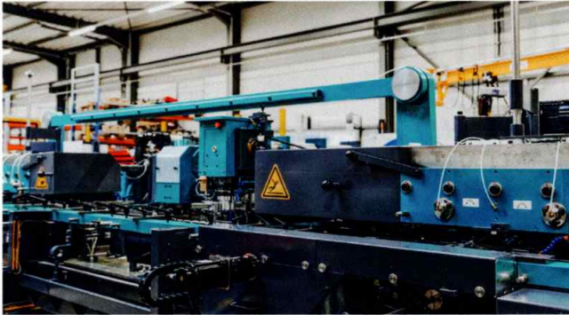
The new-generation machines produce eighty 420-mm-long, 10-mm-diameter (OD) full-thread screws per minute. © Amba
